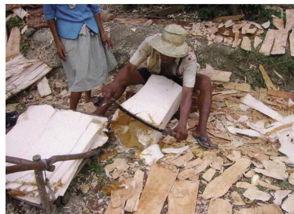
Fig. 3. Dry-extraction method for sago starch (Toyota and Okazaki, 2003)
