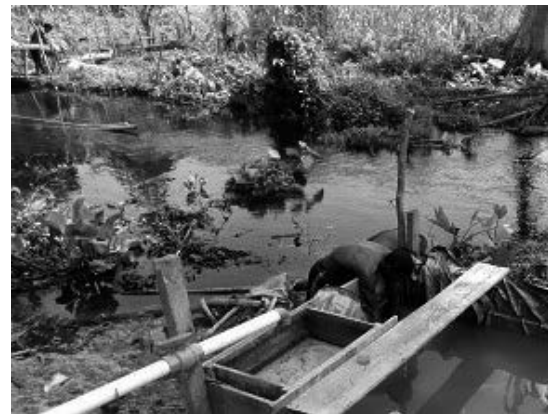
Fig. 3. Starch sedimentation tank made of wooden box covered with water proof plastic sheet.
