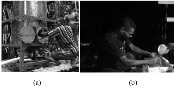
Fig. 7. Sago pith waste was discarded from the extractor tube (a) and manually extraction of 1 kg of waste sample (b).
